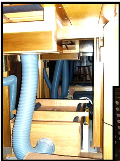
Chancel Division reservoir and Great I/Positiv underside of pipe chest
