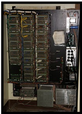
Allen digital computer to play the pipe organ
